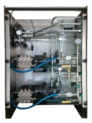
This hydraulic high pressure washer includes two high pressure water pumps which delivers 40l/min each at 140 bar. Piping and cabinet is made of stainless steel. Seethrough splash guard in front.
